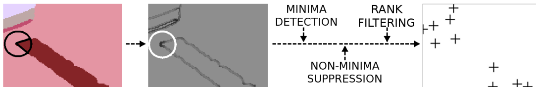
Figure 2.3: Extraction of interest points from segments with SUSAN .
