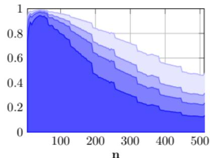
(Top) CPU. (Bottom) GPU. The fraction of time spent in copies/transpositions. Lines are shown with 1, 2, 3, and 6 transpositions.
